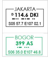
VOR / VORDME or VORTAC identification component, with frequency, identifier, and Morse Code & coordinates. DME capability is indicated by a small "D" preceding the VOR frequency at frequency paired navaids. VOR and VORTAC navaid operational ranges are identified (when known). On High/Low altitude Enroute Charts, geographical coordinates (latitude and longitude) are shown for navaids forming high or all altitude airways and routes.
